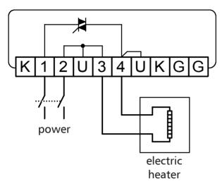
Connection of the PULSER controller to an HDE ducted electric heater and a TG-K330 external ducted air temperature sensor
